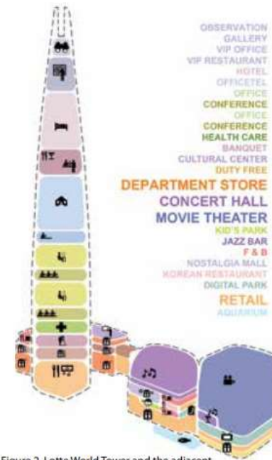
Figure 2. Lotte World Tower and the adjacent podium incorporate a tremendous density and diversity of programming.
